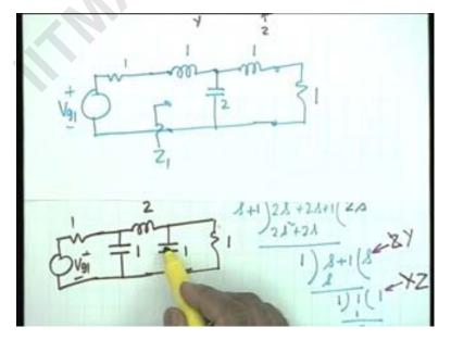
if we take s one one s as equal to minus s cube divided by s cube plus two s squared plus two s plus one then your impedance Z one shall be equal to one plus this one plus s one one divided by one minus s one one
