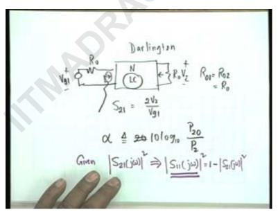
two synthesize an LC two port which is terminated in equal resistances let's say R zero and R zero and we took R zero R zero can be normalized to one ((ohm)) (00:01:12) if you so desire both terminations are equal
