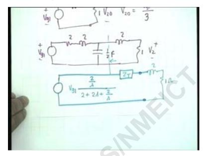
to solve this network as for as IVR is concerned IVR is simply found out Vg one two ohms to find out V two zero you simply connect the load here one this voltage will be V two zero and obviously V two zero is equal to Vg one divided by three agree
