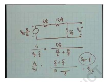
what do i get i get Vg one five by six open circuit voltage five ohms divided by five plus one six and what is the equivalent resistance of five ohms and one ohms yes five by six then i had ten by nine okay and five by six this is V two
