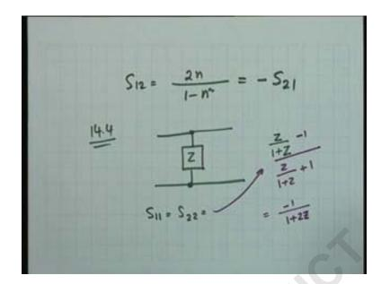
therefore S one two is equal to twice n divided by one minus n squared which is exactly  $\langle a\_side \rangle$  ((S two))  $\langle a\_side \rangle$  minus S two which shows the non reciprocal nature of the device okay
