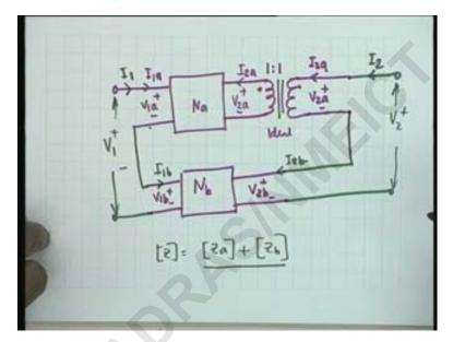
that is in general our network would be like this Na and instead of connecting directly we shall use a one is to one ideal transformer one is to one ideal transformer
