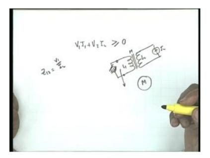
V1 II plus V2 I2 it is greater than equal to 0. For an ideal transformer, it is exactly equal to 0 for a non ideal transformer it may be greater than 0 a transformer is a passive device all right. The last problem of the day.
