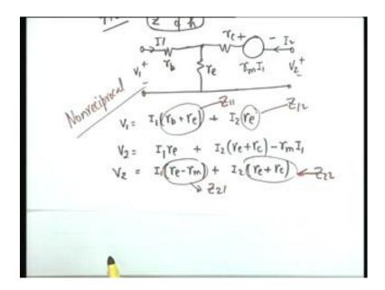
I shall, speak out the problem; the problem is to find z and h parameters of the common ammeter transistor, represented by it is T circuit model. The model is the resistance rb, resistance re, then a resistance rc. Then a voltage generator with this polarity rm times I1 and this is the 2 port V2, I2, V1, I1 to find the z and h parameters of this 2 port, which represents the equivalent circuit of a common ammeter transistor.
