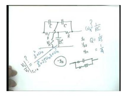
You have an R, you have an R then a C and then here the 2C I am specializing the values. And then you have a C and C in parallel with not 2R; R by 2 the parallel combination of R and R. Parallel combination of C and C is here a parallel combination R and R is here. It is instruct to you to find out the parameters Y11 Y22 and Y12. And you shall notice that minus Y12 parameter of this circuit shall look like this.
