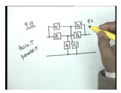
We go to the last problem of the previous session that is: 9.13. And the 9.13 says find the Y parameters of the twin-T circuit of problem 9 2c. Well problem 9 2c had 2T networks in parallel. So, it is called a twin-T. The circuit is of this form Z1 Z2 Z3 this is 1 of T's.
