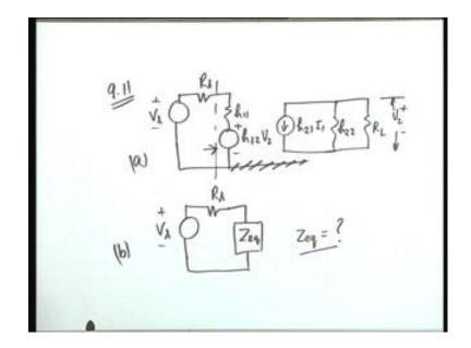
This is also from the previous set problem set 6 9 11 says: the circuit in part a of figure part a is this. We have a Vs Rs h11 this is in terms of h parameters plus minus h12 V2 no there is no common connection. The other part is h21 I1 then h22 then RL and this voltage is V2. This is part a of the figure the circuit in part a of the figure is to be described by an equivalent input circuits shown in part b Part b is Vs then Rs same as this and then a Zeq all right.
