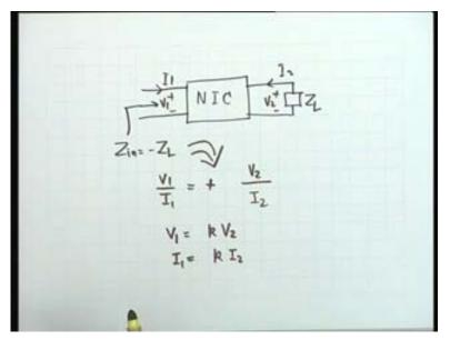
The NIC has the property that the impedance at the input is the negative of the impedance of the terminating impedance. Let us write it again, z in equal to minus z L. Now if I indicate the voltage is in currents, this is V 1 I 1 and V 2 I 2, you notice that z in is V 1 by I 1 minus z L is V 2 by by I 2, no. The relation between V 2 and I 2 is V 2 is equal to minus I 2 z L, is not that right? because the directions not agree and therefore the sign of the plus, is that okay?
