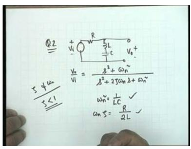
Question number 2 is, the first part was absolutely simple, there is no problem in this, L and C, there are no special values, this is V 0. The question was; in the network shown below write an expression for the transfer function, that is, v 0 by V i and I wanted in terms of zeta and omega n, zeta and omega n and I also stated that zeta is less than 1. There were questions 7
