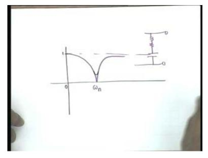
It must start at 1 and end at 1. Also, it is obvious that at omega equal to omega n, the value is 0. So the minimum value is 0, at omega equal to omega n and the maximum value is 1 occurring at 0, as well as at infinity. This is the magnitude for it. Yes, any question?
