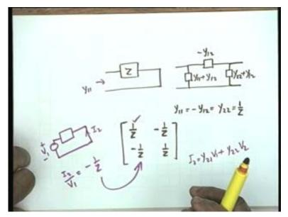
On the other hand, if I want to find out the y parameters of this, I will first find the easy way out. The easy way out is, you recall the equivalent circuit, pi equivalent circuit, which are in terms of the y parameters and this is y 2 2 plus y 1 2. By comparison, you notice that y 1 1 plus y 1 2 is equal to?
