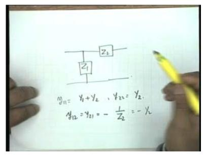
Now let us look at the y parameters. Once again the network is z 1 and z 2. Let us do it in 1 or 2 different ways, y 1 1 if I apply the definition, short circuit this and then measure the input admittance, obviously, this will be y 1 plus y 2, where y 1 is 1 by z 1, y 2 is 1 by z 2, y 2 2, if I measure here with this shorted, obviously, this will be simply y 2 2. Now can anybody tell me what would be y 1 2, without any calculation?
