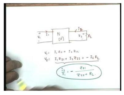
I have the network N, V 1 I 1 V 2 I 2 and there is a termination R L, so I write the equations N has been described by its z parameters, so I write the equations V 1 equal to I 1 z 1 1 plus I 2 z 1 2. There should have been an objection to T parameter equivalent circuit which none of you raised.
