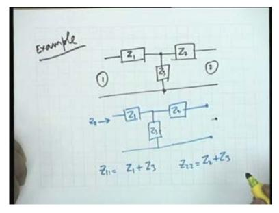
Let say z A, let us take z 1 z 2 and z 3. This is port 1 and this is port 2. We are required to find out the z parameters of this circuit. One of the ways is go back to definition, whenever in doubt go back to the rules. Let us apply the definition, z 1 1, as you know, is the driving point impedance at port 1 with port 2 opened. If this is kept open, then obviously, z 1 1 is simply equal to z 1 plus z 3 agreed?
