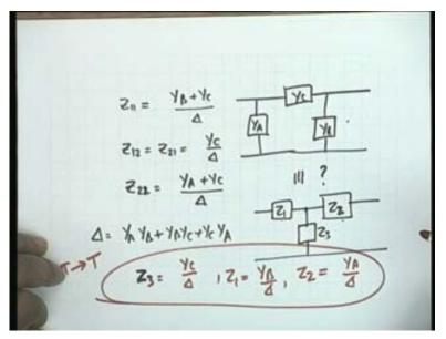
z 1 1 is Y B plus Y C divided by del, z 1 2 equal to z 2 1 is equal to Y C divided by del and z 2 1, I am sorry, z 2 2 would be Y A plus Y C divided by del. This is what is the network? Let me draw the network. Network is, we have a Y A, we have Y C and we have a Y B. What is del? The determinant of the, determinant of the, it is Y A plus Y C multiplied by Y B plus Y C minus Y C square. So it is simply Y A Y B, it a cyclic summation of products, Y B Y C plus Y C Y A.
