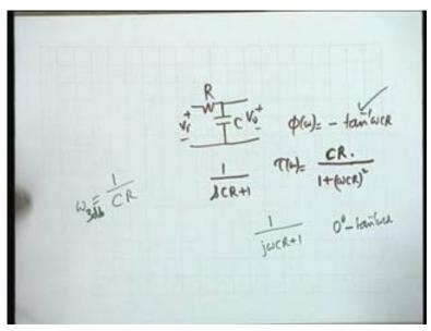
You can easily verify that any of these networks, simple networks, for example, R and C, the low past filter. What is the phase phi? Omega is equal to, well what is the transfer function of this? S C R plus 1. So if you put S is equal to j omega, this is the input and this is the output, so phi omega is minus tan inverse omega C R and therefore, tau omega is negative gradient of the phase. So it would be 1 by 1 plus omega C R whole square. Is that okay?
