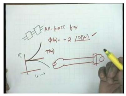
Sir: That is right and therefore, for an all pass network function, phi omega would be equal to minus twice angle of D j omega. Is that clear? Minus twice angle of D j omega. Angle of, minus
