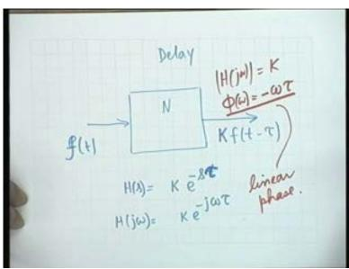
Suppose we have a network N and let us say, it is excited by, we are not showing a voltage or current, is excited by an input, let us say e of t, make it f of t where the f can be a voltage or it can also be a current and let the output be delayed by an amount tau. Let the network N be such, let the output is exactly of the same wave shape f, but it is delayed by tau. In addition, the network N may either amplify or attenuate the signal, so we put a constant K.
