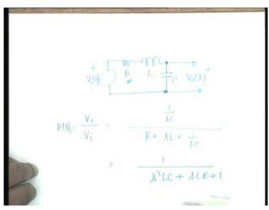
Now let us look at this circuit. We have a single tuned circuit, is a resistance, inductance in series, there are various forms. We take a typical form and a capacitor C. This is my transform of the input voltage and this is my output voltage V 0 s. This is a typical single tuned circuit. The
