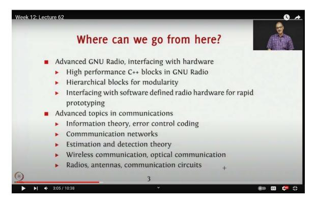
Another important topic is the use of hierarchical blocks in GNU Radio, which enhances modularity and efficiency in your projects. For simplicity, when constructing our GNU Radio flow graphs, we often included all components within the same graph. This approach sometimes led to very large graphs with repetitive elements. For instance, in cases involving modulation and error control coding, I had to duplicate certain blocks to compare uncoded versus coded scenarios, which led to some redundancy.
