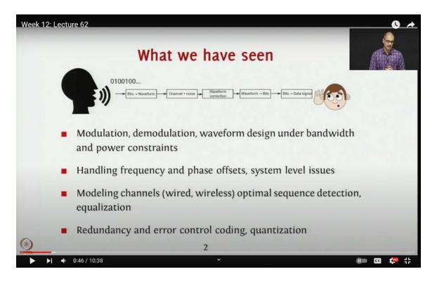
We began by exploring the conversion process from bits to waveforms. We examined how real signals can be translated into bits and then how these bits can be converted back into waveforms. This included studying modulation techniques and waveform design while adhering to bandwidth and power constraints. These constraints are critical since practical communication channels have limited frequency ranges and power limitations that must be respected for effective communication.
