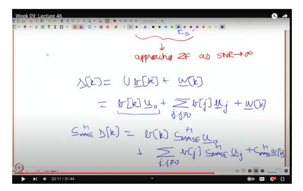
In high SNR conditions, the MMSE equalizer behaves like a ZF equalizer, whereas in low SNR conditions, it avoids blindly inverting the channel, which would otherwise amplify the noise. Instead, it strikes a trade-off to achieve the minimum mean squared error, which, we hope, results in better performance.
