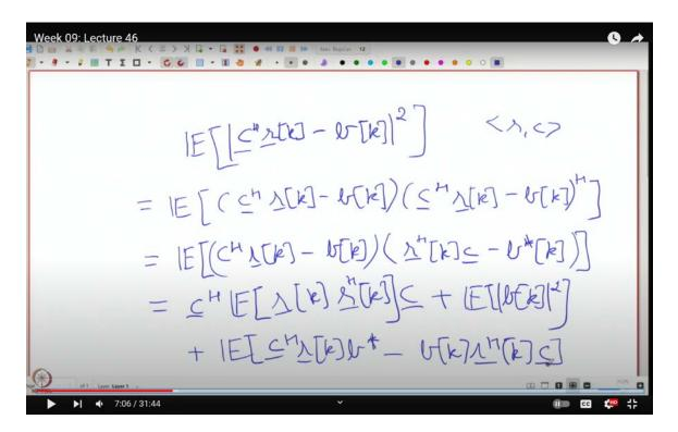
Similar to other methods that involve minimizing squared error, the use of squared error in MMSE allows for a straightforward computation of the equalizer. By differentiating the squared error with respect to the filter coefficients and setting the result to zero, we can derive the filter coefficients. This is precisely what we will examine in this lecture.
