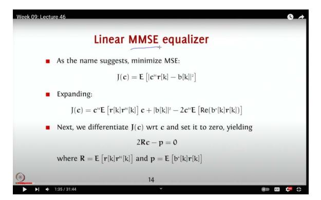
However, as we observed both in our theoretical discussions and through GNU Radio simulations, zero-forcing comes with a significant drawback: it can lead to substantial noise enhancement. This noise enhancement is particularly detrimental when operating in environments with low signal-to-noise ratios (SNR). Consequently, the zero-forcing equalizer may not be the best choice in scenarios where the SNR is very low.
