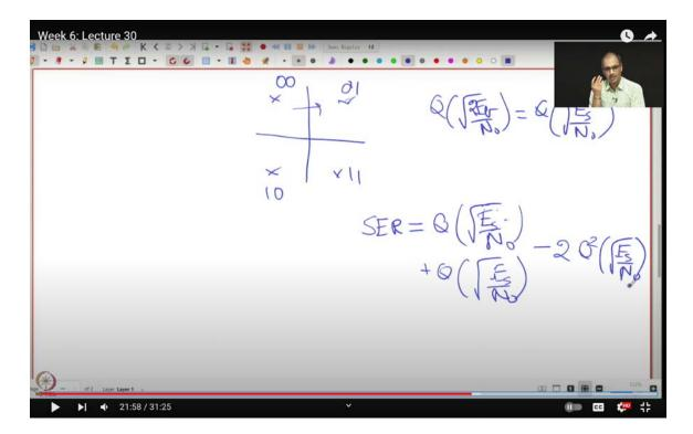
To calculate the BER for PAM-4, the approach is somewhat similar to that of BPSK, but with a slight complexity. The issue arises because you need to calculate the BER separately for different pairs of symbols. For instance, consider the transition from 00 to 01. To
