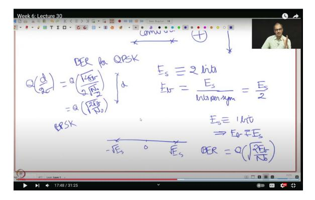
Thus, the bit error rate for BPSK can be expressed as  $Q\left(\sqrt{\frac{2E_b}{N_0}}\right)$ . This is because, in BPSK, a symbol error directly results in a bit error, making the symbol error rate and bit error rate equivalent.
