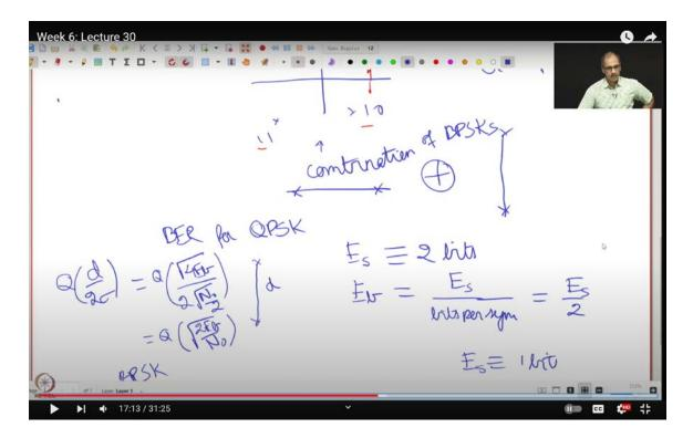
So, let's proceed by considering QPSK as a combination of BPSKs. Now, let's compute the bit error rate for QAM-4, or equivalently, QPSK. But before we dive into that, there's an important concept we need to address: bit energy.
