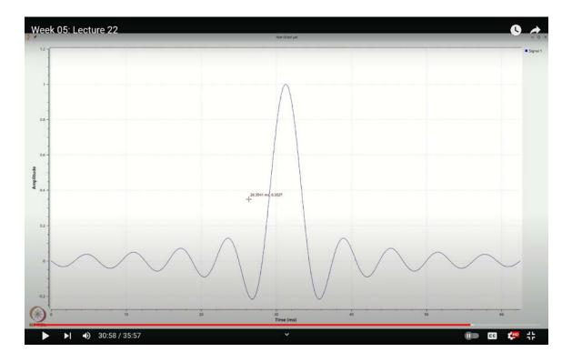
Now, execute the flow graph. Save and run it, and you will see the sync signal varying. The variation occurs because the width of the time sync and the sync signal are not the same. To correct this, ensure that the time sync block is configured to display the sync signal fully. Double-click on the time sync block and adjust its settings.
