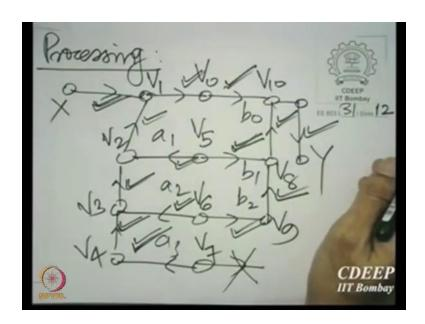
Now, let us translate this reduce signal flow graph into a sequence of steps. Now, what we need to do is to identify what are called the 1st level nodes that is nodes which can be calculated first, nodes which can be calculated next and so on, step by step. So, once we have a signal flow graph like this, we have to identify the effective source nodes in the signal flow graphs you begin from the source and go to the sink that is a universal rule.
