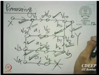
So, that leads us to the step of preparation for the next input. How do we prepare for the next input look at the string of delays, the string of delays would take you from  $V_0$  to  $V_5$ ,  $V_5$  to  $V_6$ ,  $V_6$  to  $V_7$ . And in this string, this one is the last delay and therefore you need to put at  $V_7$  what you had at  $V_6$ . This is operated first, you need to put at  $V_6$  what you have at  $V_5$  and you need to put at  $V_5$  what you have at  $V_0$ .
