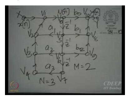
Now, you see having drawn a signal flow graph, the next task is to realize that signal flow graph in the form of an algorithm or in the form of what is called pseudo assembly language or pseudo code. We need to be able to program structures, we cannot be satisfied simply with drawing them. So, to program the structure, we need to evolve what is called a generic loop.
