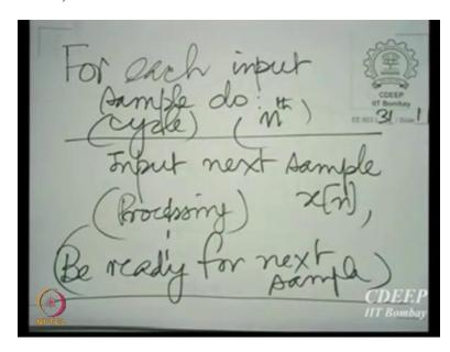
So, this is the generic loop that you would require to realize that signal flow graph for each input sample, do all the following that is the in the nth sampling cycle, input the next sample, let us call it x[n] carry out some kind of processing and be ready for the next input sample to come, that means at the end, so there is a loop operating for every input sample here.
