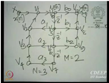
So, let us again take the same signal flow graph, and let us evolve a process to write down a pseudo code for that signal flow graph. So, let us flashback that signal flow graph for you. Now, the rule is very simple, you see, what really are delays. Delays, as you see here are mechanisms for preparing yourself for the next sample.
