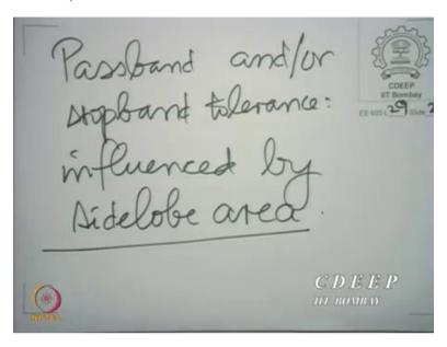
The passband and stopband tolerance influenced by side lobe area. The reason for this is simple. The tolerance is caused by side bands entering and leaving the ideal pass band in the periodic convolution between the ideal DTFT or the ideal frequency response and the windows spectrum for the pass band is the region where the main lobe has completely entered the ideal passband and now the side lobes are entering and leaving.
