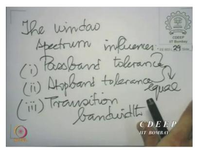
The passband tolerance, the stopband tolerance and the transition band or transition bandwidths from the window approach we do not have separate control on the passband and
