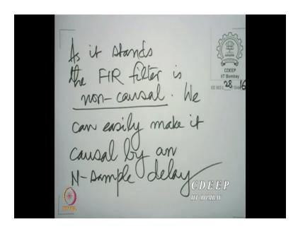
You know, if as it stands, the FIR filter is non-causal. But it is very easy to make it causal. All that you need to do is to delay the output by N samples. We can easily make it causal by an N sample delay. And N sample delay is very easy to understand in the frequency domain. All that N sample delay does is to impose an additional linear phase.
