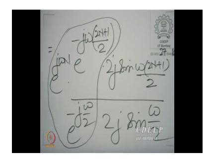
Common ratio,  $e^{-j\omega}$ , first term or leading term  $e^{j\omega N}$ . And that is  $e^{j\omega N} \frac{\left(1-e^{-j\omega(2N+1)}\right)}{\left(1-e^{-j\omega}\right)}$ , this is the sum. Now, we can do a little bit of work to get this in the form of a *sin* by a *sin*.
