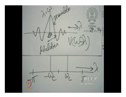
Now, what I shall do is to make the window spectrum and to do that, it is much easier for us to draw the window spectrum on a separate sheet of paper. We will exaggerate it by drawing the
