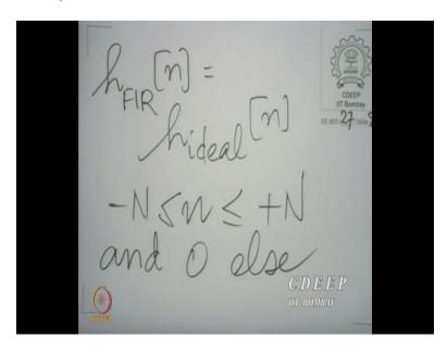
So, clearly,  $h_{FIR}[n]$  is  $h_{ideal}[n]$ , for n between -N and +N and 0 else, is the obvious way to do it. Retain the samples from -N to +N, throw away the rest. Now, this is equivalent to multiplying the ideal impulse response via the function which is I between -N and +N, and +N0 outside.
