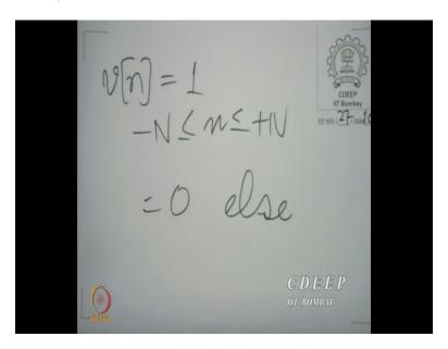
So, v[n] in this case is equal to I, for n between + N and - N and,  $\theta$  else, that is obvious. So, multiplies by a function which is I in the range where you are retaining the samples and by  $\theta$  in the range where you are throwing away the sample, that is an obvious. Now, why this approach or why this perspective is useful to us is because it immediately gives us a clue how we can identify the scars that are produced in this truncation.
