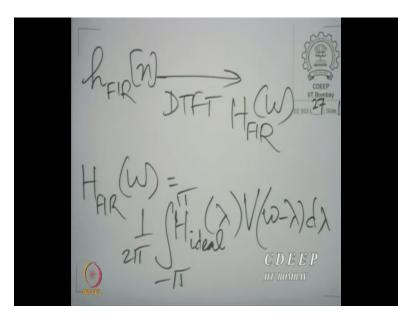
And obviously, the discrete time fourier transform of  $h_{FIR}[n]$  which, we shall in a minute denote by  $H_{FIR}[\omega]$ , is given as follows,  $H_{FIR}[\omega]$  is, as we know,  $\frac{1}{2\pi}\int$  over a contiguous range of  $\pi$ , we could choose the principal interval  $-\pi$  to  $\pi$ . Well, you know, we had a choice, we could either move V or we could move  $H_{ideal}$ .
