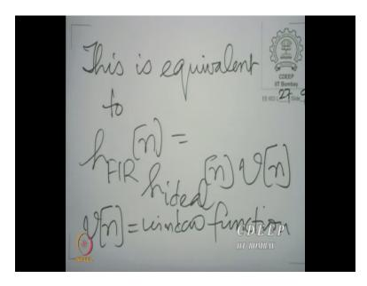
So, this is equivalent to  $h_{FIR}[n] = h_{ideal}[n]v[n]$ , v[n] is called a window function. I used v instead of w for window, w is likely to be confused with  $\omega$  and I do not want to use w for that reason. So, we will use v.
