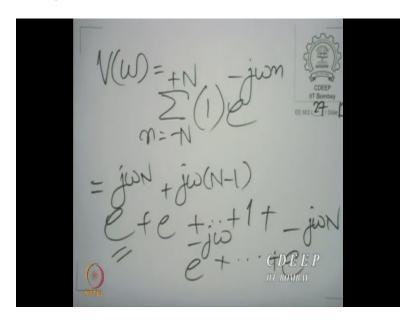
So,  $V(\omega)$  looks like this. It is a discrete time fourier transform,  $\sum_{n=-N}^{+N} (1)$ , that is the value of V[n] in that region and 0 outside,  $e^{-j\omega n}$ . Now, we can expand this. It is  $e^{j\omega N} + e^{j\omega(N-1)} + ... + 1 + e^{j\omega} + ... + e^{-j\omega N}$ .
