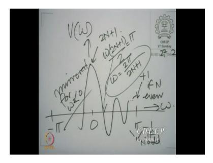
$V(\omega)$  is going to show a pattern like this, this time I go out all the way from  $-\pi$  to  $\pi$ . It is going to have its, what is called the main lobe and then it is going to have a decreasing character. So, it will either end this way or this way. Now, +1 if N even, and at -1 if N odd and mirrored on this side.
