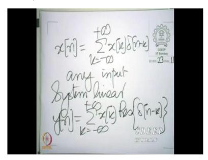
Now, you see when a system linear of course any input can be written in terms of the impulses. This is true for any input and this system is still linear. Then one thing is clear
