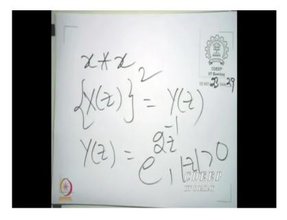
And that is easy to do because when you convolve, when you convolve the sequence x with itself with z transform is multiplied. So, you get Y(z); and therefore Y(z) is simply  $e^{2z^{-1}}$ , with the same region of convergence; |z| > 0 and just as you can expand  $e^{z^{-1}}$ , you can also expand  $e^{2z^{-1}}$ ; that is very easy to do.
