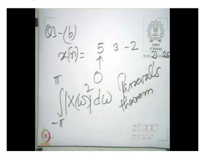
Now, question 3 b give you the sequence x[n]; this is the sequence was given and you are required to evaluate  $\int_{-\pi}^{\pi} |X(\omega)|^2 d\omega$  of course This is easy to do; one can use the Parseval's theorem for doing it.
