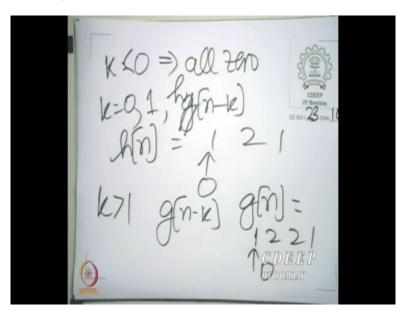
K < 0 all 0, k = 0,1 its g [n-k]; and g[n], I am sorry h [n-k]; and h[n] is specified to be 1 2 1 with this 1 placed at 0. and for k > 1 its g[n-k] and g[n] is specified to be 1 2 2 1 with this 1 located at 0. So, the first question is to write down the output y[n] in terms of the input x[n] in general.
