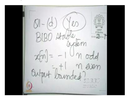
So, question 1d was if you give the BIBO stable system, the input x[n] = -1, for n odd; and 1 for even n is the output bounded and of course the answer is yes; that's because the BIBO stable system, the input is bounded by 1 and therefore the output must be bounded. So That is simple.
