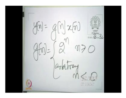
So, indeed y[n] = g[n] x[n]; where g[n] is clearly specified to be  $2^n$ , for  $n \ge 0$ ; an arbitrary for n < 0. You can of course extend it to  $2^n$  and also for n < 0; it doesn't matter.
