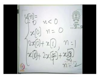
This is the response that you get y[n] = 0 for n < 0. x[0] for n = 0, 2x[0] + x[1], for n = 1. So, you can expand this, you can expand this output and get; so I am just putting down the response. X[1] + 2x[2] + x[3], for I am sorry; X[1] + 2x[1] + x[2], for n = 2 and we can continue this.
