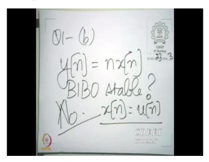
Question 1 part 2, part b asked whether  $y[n] = n \ x[n]$  is a bounded input bounded output stable system? And the answer is no. That's because you could give a counter example by taking y[n] = u[n], this is bounded. But, the output is clearly unbounded, so you have bounded input, you can have unbounded output; and that is how it serves as a counter example. If there are any questions please post them right then and there.
