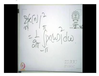
Because, you know that  $|x[n]|^2$  some there were all n is  $\frac{1}{2\pi} \int_{-\pi}^{\pi} |X(\omega)|^2 d\omega$ . So, the idea was that without without evaluating the discrete time Fourier transform; you are required to find this quantity. Which is easy to do because you can take  $\pi$ to the other side, we are done.
