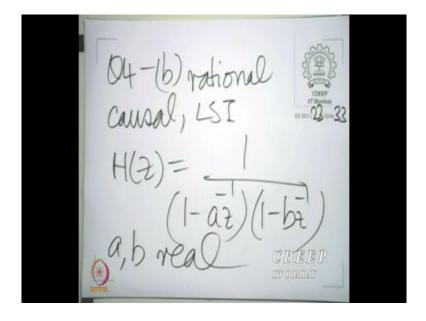
And there you are told that there is a system given to you; it is a rational causal LSI system and the system function was given to you  $H(z) = 1 \frac{1}{(1-az^{-1})(1-bz^{-1})}$ ; and a and b are real constants. You do not know whether a and b are equal or not equal, but you know that they are real.
