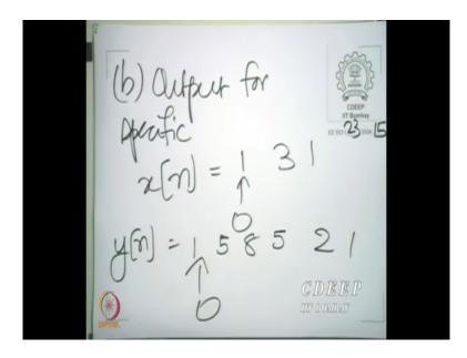
And the specific input was this and of course one can simply substitute and one can get the following expression. So, this is for specific input, if one just substitutes the values of x[0], x[1], x[2]; and puts them in the respective samples to get the output.
