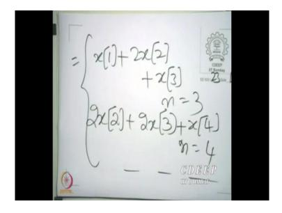
It is equal to x[1] + 2x[2] + x[3], for n = 3; 2x[2] + 2x[3] + x[4]. So, you see it is clearly shift variant, the behavior changes for n = 4 and again for n = 5, we need to write a separate expression; and beyond that you can write a common expression.
