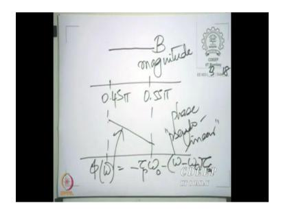
And you are given the magnitude in the range  $0.45\pi$ , you see the magnitude between point. You are only given the magnitude between 0.45 and  $0.55\pi$  and you are told the magnitude is constant at B, and now told that the phase is essentially a linear phase. If not one one call would not call it linear, actually, one should call it pseudo linear. Pseudo linear because it does have straight line expression, but it does not pass through the origin.
