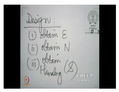
Design means the following: obtain E, obtain N, and then obtain therefore obtain  $H_{analog}(S)$  And how would you obtain  $H_{analog}(S)$ ? You would have to identify the poles and then segregate those poles that correspond to  $H_{analog}(S)$ , by removing the poles that correspond to  $H_{analog}(S)$ . So, let us obtain E first, E is very easy.
