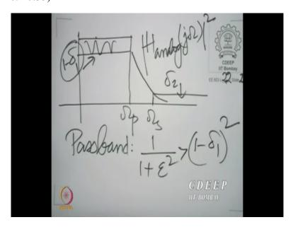
You see, it is very clear that there would be an oscillatory behavior in the passband. I am plotting  $|H_{analog}(j\Omega)|^2$ , and then from the edge of the passband; and downwards there would be
