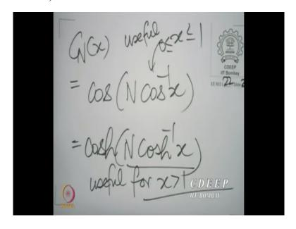
The same  $C_N$  (x) can be written as  $cos(N cos^{-1} x) = cosh(N cosh^{-1}x)$ . This is useful for x between 0 and 1; because then  $cos^{-1} x$  becomes real. And this is useful when x > 1, because cosh for a real argument is always greater than 1, greater than or equal to 1. Cosh x for real x is of course an even function; so cosh of x is equal to cosh of minus x. And therefore, we need only to look at the positive side of x.
