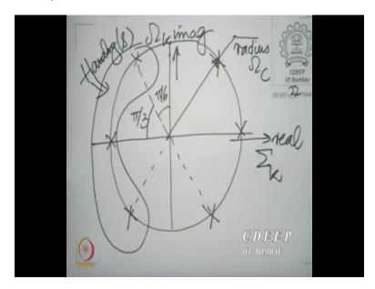
And all that we need to do now to identify  $H_{analog}(s)$  is to take away the poles in the left half plane. So, these poles, these three poles give us the poles corresponding to  $H_{analog}(s)$ ; and therefore of course naturally these three poles are the poles corresponding to  $H_{analog}(-s)$ . Now, you see let us write down therefore the system function corresponding to  $H_{analog}(s)$ .
