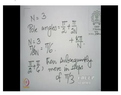
So, for the case n equal to 3, let us write down the angles, pole angles. The pole angles are of course given by  $\pi$  by 2 plus  $\pi$  by 2N, plus k  $\pi$  by N. And if N is equal to 3, then  $\pi$  by 2N is  $\pi$  by 6. So, you can of course you see all that you need to do is to identify that there are 2N distinct poles here.
