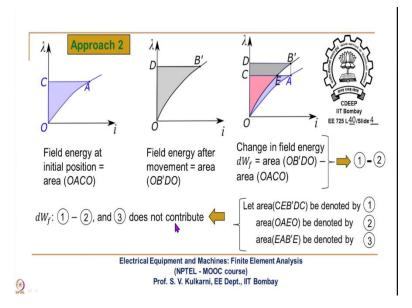
In approach 2, we are keeping current as constant. Here, the characteristics changes from AB' as shown in the following figure.
