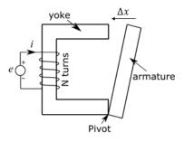
Once the current is passed through the coil the armature will get attracted. Suppose if the armature is moved by a small distance  $\Delta x$  in the *x* direction (indicated in the above figure) then the operating point in the following characteristics would shift from A to B.
