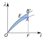
The value of co-energy is represented by the shaded area in the above figure. The same is observed in the two simulations given in the above slide. The value of force is calculated as  $2.28 \times 10^4$
