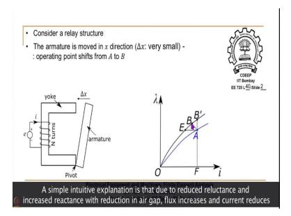
Now, consider a relay structure shown in the following figure with a hinged armature supported by a pivot.
