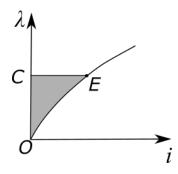
The field energy at the initial position corresponds to the area of OACO highlighted in the previous figure. Field energy after the movement of  $\Delta x$  is represented by OECO area. So, the change in field energy  $(dW_f)$  will be the difference in the two areas. Remember that the field energies are calculated by using  $\int i d\lambda$ . So,  $\int i d\lambda$  is the field energy and it is equivalent to  $\int H dB$  because *i* correspond to H and  $\lambda$  corresponds to B.
