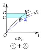
So, the area in sky blue color is representing  $id\lambda$  and its value is equal to area 1 + area 3. The change in field energy  $dW_f$  is area 1– area 2 as seen in the previous slide.
