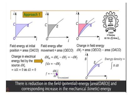
Let us see the two approaches in detail. The first approach is constant flux condition. The characteristics shown in the following figure is for the initial position of the armatures and A is the operating point of the magnetic circuit in this position.
