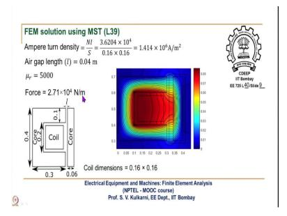
In L39, we have already calculated the force using the MST approach. In the above slide, we have shown the calculations again and the value of force calculated by using this method is  $2.71 \times 10^4$  N/m.
