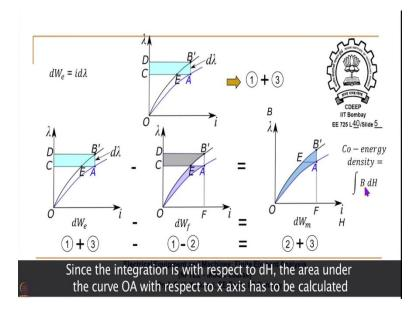
Earlier we have seen that  $dW_e = id\lambda$ . So, once we move from A to B' as shown in the following figure then the electrical input has increased.
