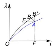
So, initially, if the characteristic curve OA corresponds to a particular gap and after that if the armature is moved by  $\Delta x$  then the operating point shifts on the curve OEBB' through the line AB.
