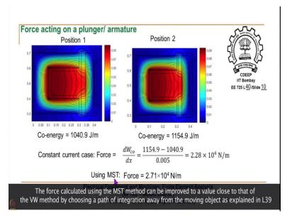
Now, we will calculate the force using the co-energy approach which is nothing but virtual work method. So, in the above slide flux plots of two FEM simulations are shown. The flux plot on the left hand side is for position 1 with higher distance and the second figure is the solution for
