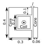
The magnetic circuit has a C shaped core and an armature which is hinged. The armature is free to move. The moment we pass the current through the coil the core will attract the armature. In this circuit, we have considered the length of the air gap as 0.04 m. There are two air gaps in the circuit and the total reluctance of the magnetic circuit is given by
