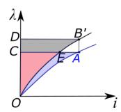
So, at the initial position, the operating point of the magnetic circuit is A, then we went to operating point B' after a movement of  $\Delta x$ . The field energy at the initial position is represented by OACO and field energy after the movement of  $\Delta x$  is equal to the area OB'DO. So, the change in field energy is the difference between the two areas OB'DO and OACO as indicated in the above figure.
