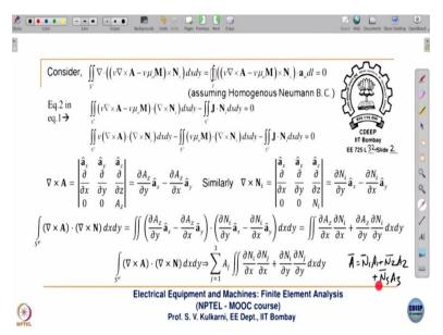
For  $\mathbf{A} = \mathbf{N}_1 A_1 + \mathbf{N}_2 A_2 + \mathbf{N}_3 A_3$ , **A** on the left hand side is a vector so on the right-hand side also there has to be a vector, but  $A_1$ ,  $A_2$ , and  $A_3$  are just the scalar magnitudes. So, here **A** being a vector should get reflected by  $\mathbf{N}_1$ ,  $\mathbf{N}_2$ , and  $\mathbf{N}_3$  being vectors.
