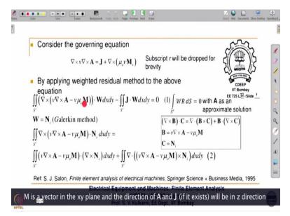
But here, M is a vector in xy plane and its direction is not along z direction, so we have to develop the formulation in vector notation. So, that is why the weighting function is also a vector because residue is a vector. So, now, we are considering Galerkin's approach and we took the weighting function as shape function and the only difference is both functions are vectors.
