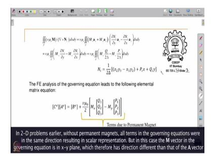
But here we are developing vector formulation because  $\mathbf{M}$  will have two components (*x* and *y* components) as we see later.
