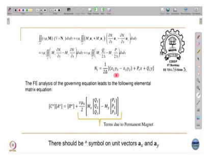
The function  $N_i$  is our standard shape function. As we discussed earlier the shape function was in z direction because A was in z direction. So,  $N_i$  was in z and it was a function of x and y.
