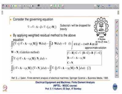
So, the above integral goes to 0 if there is a homogeneous Neumann condition on the outermost boundary. So, now we are left with the following term.
