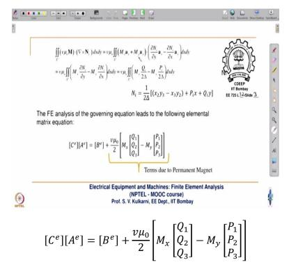
The  $[B^e]$  matrix in the above equation is our standard matrix which will come from a current source condition. That means if there is J in the problem domain then the entries of  $[B^e]$  matrix will be  $J\Delta/3$ . When we combine all the element coefficient matrices then at the end if there is a non homogeneous condition, it will lead to a boundary condition matrix which will come on account of the following integral
