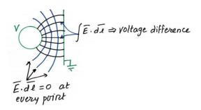
You have these equipotential lines as shown by the blue contours. And then you have the locus of electric field intensity vectors given by the black contours. The  $\int \mathbf{E} \cdot d\mathbf{l}$ , along any of the field contours gives the voltage difference between the two electrodes.
