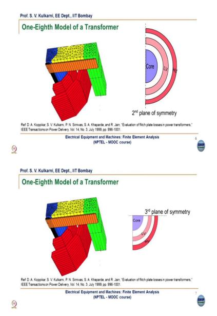
Second symmetry is on the vertical plane of the coils and the third symmetry is on the other side of the coils. So, the coil is modeled only one fourth along the  $\phi$  direction. So, it is a quarter model along the  $\phi$  direction because we are exploiting the field symmetry at the two points separated by 90 degrees along the  $\phi$  direction.
