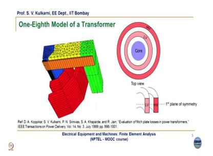
Now, this is another example to show how do we reduce the complexity. In the above slide, a section of a large power transformer is shown, here what is done is, although as you can see again here, there is no Cylindrical symmetry at all, because, around this axis of the coil, the core is not symmetrical, and the core is more or less a planar structure so there is no Cylindrical symmetry.
