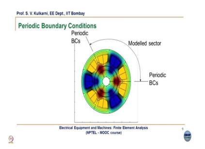
So, you do not have to model the entire 360 degrees geometry. You can model only a sector and then impose what are known as periodic boundary conditions and in the post processing stage, you will get the entire field distribution. How do we do that? There will be a separate lecture in this course on how to use periodic boundary conditions and improve the analysis, that we will see later.
