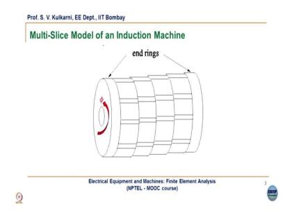
But even when you use Cartesian system, you can do some approximations like what is shown in the above slide. For example, in the figure, the rotor structure of a Squirrel Cage Induction motor with skewed rotor bars is shown. Now of course, what is shown here is a multi-slice model since the induction motor is with a skew of some finite angle, so it becomes a 3dimensional analysis, but what you generally do here is you divide this model into a number of slices.
