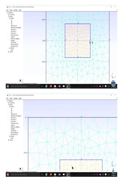
In the above two slides, more or less all elements are equilateral triangles and they are equally spaced. Also, the elements in two sub-regions are with different colors. Now, here we want to highlight one more point. In case of electrostatic problems, there is no need to mesh the geometry that corresponds to the conductor because E field is 0 in that region. So there is no need to calculate the potential values in that region.
