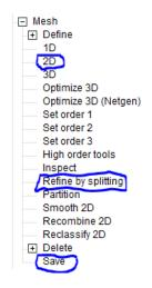
Since the problem domain is a 2D geometry, click on 2D to generate mesh which is shown in the above slide, but this is a very coarse mesh. Now you need to refine this mesh, for that you click on refine mesh. By this you can generate a refined mesh as shown in the following slide.
