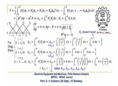
The functional for Poisson's equation is modified as given below by substituting the general expression for  $\phi$ .
