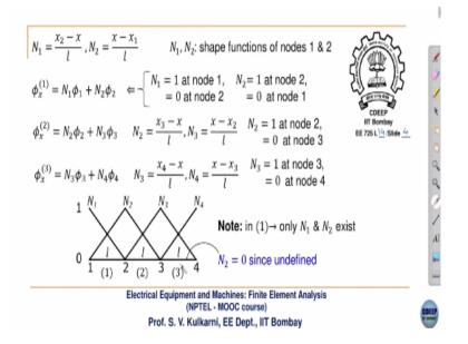
Now, what are these  $N_1$  and  $N_2$ ?  $N_1$  and  $N_2$  are the shape functions of nodes 1 and 2. What are their properties? You can see  $N_1 = 1$  at node number 1 and it is equal to 0 at node number 2. You can verify that by substituting the coordinate of  $x_1$  in the expression of  $N_1$ , it will be equal to 1 as given below
