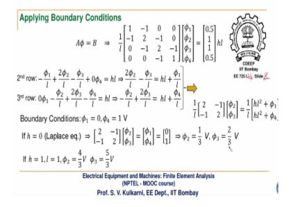
$A\phi = B$  is the final matrix equation. Now, we impose the boundary conditions which are in terms of  $\phi_1$  and  $\phi_4$ . The boundary conditions for this problem are  $\phi_1 = 0$  and  $\phi_4 = 1 V$ . Now, to apply these boundary conditions, we are expanding the second and third rows of the matrix equation  $A\phi = B$  as given below.
