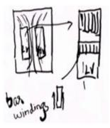
In the figure on the left side, the outer boundary is the boundary of a core window, also you have 2 windings (LV and HV) and leakage field indicated with black lines as shown in the figure.
