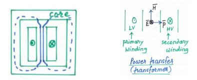
Now this is a transformer having LV and HV windings with current directions coming into and out of the plane and the corresponding leakage field will be as shown the above figure.
