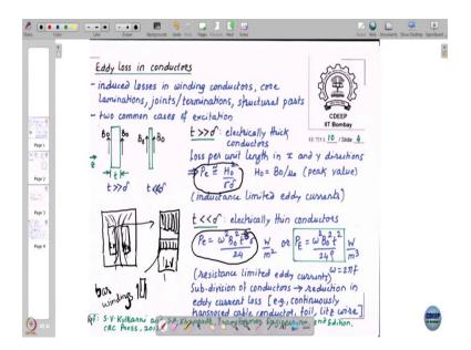
In this slide, we will derive the basic formula for induced losses in windings conductors, core laminations, joints and structural parts. There are two common cases of excitation. In the first case, the conductor is very thick and it is excited on both sides by tangential flux density ( $B_0$ ) as shown in the following figure.
