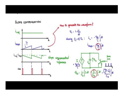
Let us now try to understand what slope compensation is and how to obtain the slope compensated reference waveform. Let us understand it with the help of some waveforms with respect to time, I will plot i L ref which is nothing but a constant dc value. So, the inductor current waveform is compared with this constant dc and then that is how the current controlled output is generated. But this has a problem for greater than 50 percent duty cycle where it will become unstable.
