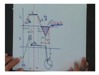
So, what I have done is that on this sheet I have just drawn the typical switching waveforms for the voltage and the current across a power diode. So, what we are doing is we are looking at both the turn on and turn off switchings of the diode. So, what you see on this side on the left side if I just draw this on the left side is a turn on and on the right side is the turn off switching of the diode.
