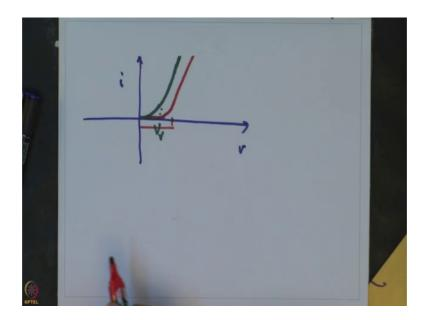
One of them is in their i v characteristics. So, one of the things that you will see is that if I draw the i v characteristic ok, of the two diodes and let us say I use a green pen to draw the characteristic i v characteristic of a signal diode. So, you can see that it actually is going to rise exponentially it drawn and there is what is called a cut in potential or contact potential and the device actually starts conducting only after that.
