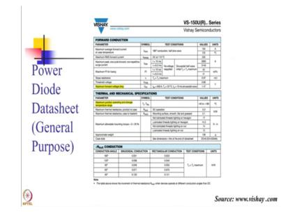
We can also see you know on this slide which is the second page of the datasheet of this particular diode the maximum forward voltage drop which actually is about 1.47 and you can see that all the other values are given at which this particular forward voltage drop will hold. So, it also gives a temperature of 25 degree centigrade it says that what is the peak current which is 600 mps and so on under those operating conditions it says that the voltage drop will be 1.47.
