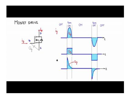
MOSFET is a very popular semiconductor switch, especially for DC-DC converter we will discuss its drive. Let me draw the MOSFET symbol. So, this is called the gate and is called the drain the substrate and the source or connected. So, you have the drain source gate, there is a natural internal body diode, the arrow here pointing to the n channel inversion layer that will get formed. So, this is an n channel MOSFET.
