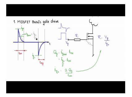
Let us now see how the basic or the fundamental gate drive for the MOSFET looks like. It is very simple it consists of only one component that is one resistor. So, let us start from the requirements the gate drive requirements, I have this timeline I have split the timeline in to the OFF state the turn ON period the ON state turn OFF period OFF state.
