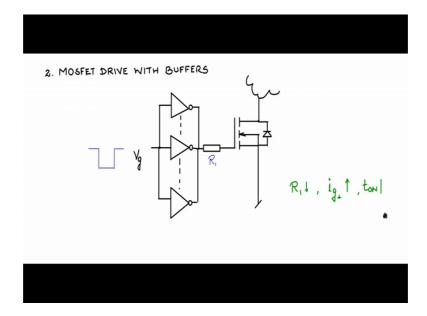
Let us discuss another MOSFET drive gate drive with buffers CMOS buffers, this can improve the turn ON speeds and turn OFF speeds. Let us see the circuit I have the MOSFET here the drain is connected to the external circuit and the drain current is what you need to control switch ON and OFF. The source as usual is connected to the ground is a Gora ground based gate drive is an internal body diode and the gate is connected to the resistor the 1 resistor gate drive.
