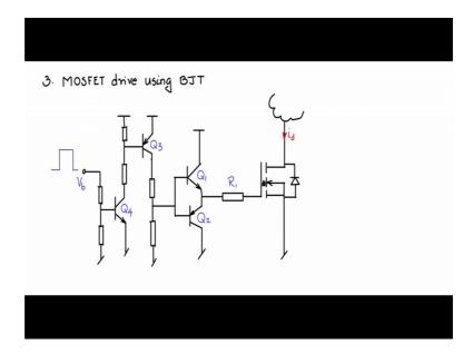
All BJT drive circuits can be used for MOSFET gate drive. Let us see an example I will draw the MOSFET, drain connected to the external load, source connected to the ground
