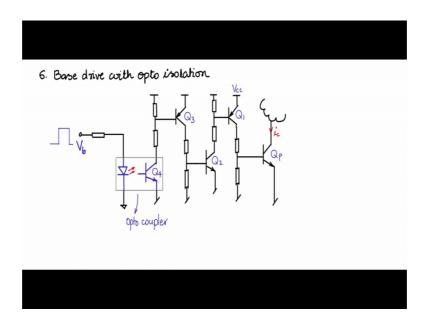
Let me now discuss another based drive isolated based drive, but instead of transformer isolation I am going to discuss opto coupler isolation; opto or the light isolation. So, let me start by drawing now here this is the power transistor Q p and that is connected to the external load the collector current of which we need to switch ON and OFF.
