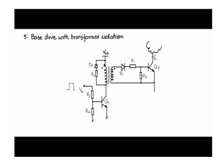
Let us now discuss a base drive circuit with transformer isolation. Let me begin by drawing an NPN transistor like this and I will drive this by a 2 resistor drive circuit. We are familiar with this kind of a 2 resistor drive circuit. We know this we know how it operates. In the collector of this NPN transistor I am going to place the primary of a coil transformer coil in this fashion call that as V cc.
