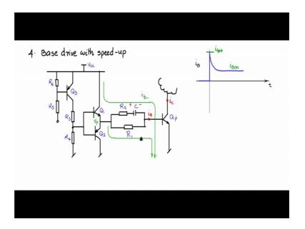
Let me now discuss another interesting Base drive circuit with speed-up; speed-up of both turn on and turnoff. Let me start with a PNP transistor, the PNP transistor the collector is connected to a resistance 2 resistance divider like this. And from the centre point of the resistance division I will pick of a point, pick of a line and then connected to the base of an NPN transistor like this.
