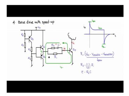
We will see that charts current starts flowing in this fashion down through like this surge flowing like this and through in this direction. So, that the base charges start recombining and comes back and completes the circuit here. So, this is the negative current. So, this is the negative current that we are seeing that needs to flow through Q p. So, that Q p turns off as fast as possible and there is base charge recombination.
