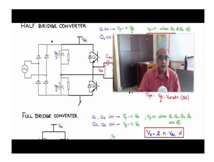
In the case of the half bridge converter and the full bridge converter you have top semiconductor switch and a bottom semiconductor switch. The bottom semiconductor switch is ground base drive, the top semiconductor switch is a floating drive. So, how do you make such kind of drives? Complimentary, but is able to address the half bridge and the full bridge converter switch arms.
