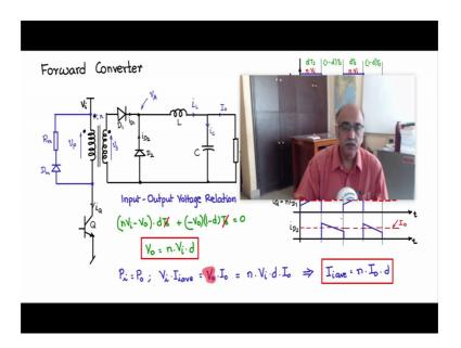
We have seen also in the forward converter there is this BJT, now we have shifted the BJT from the rail based to the ground based saying that the drive circuit is simpler if it is driving a ground based switch, we will see all those issues why it becomes simpler to drive a switch which is ground based.
