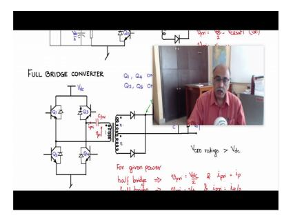
And the case of full bridge like the half bridge you have two switches semiconductor switches which are floating drive and two semiconductor switches which are ground based drive. So, these are the aspects that will come into the picture.
