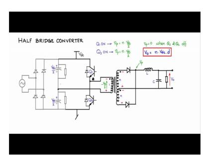
So, let us mark. So, the non dot end is positive, dot end is connected through Q 2 to ground minus so, non dot end is plus dot end minus like this. So, if we measure across the primary you have minus Vdc by 2 appearing over the primary, secondary likewise Vdc n times, V dc by 2 and n times Vdc by 2 here with the polarity are shown this diode the bottom diode is active and Vp is again seeing n times V dc by 2 just like in the push pull case.
