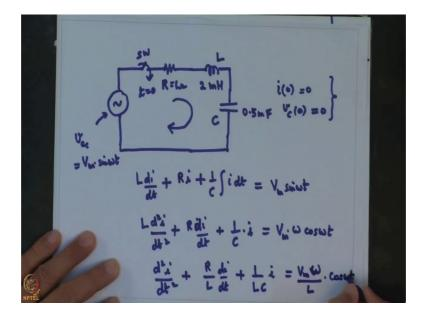
So, the EC source or the forcing function is supplying through a switch network that consists of R equal to 1 ohm an inductor which is 2 milli henry and a capacitor which is 0.5 milli farad.
