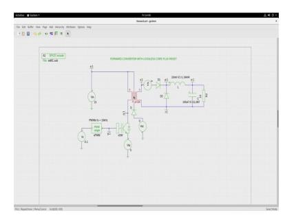
Let me now show you the simulation or the forward converter with lossless core flux reset. This is the entire circuit diagram of the forward converter with lossless core reset. Observe this transformer part so, in the transformer part you have 3 windings; one is the primary, other the secondary and in between you have the demagnetizing winding. So, this demagnetizing winding is the one which will perform the core reset. I have this demagnetizing diode flowing into the source.
