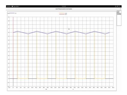
As you can see I have given it for very small number of cycles, you will see this as the output voltage v o, r ok. So, that's close to around 12 volts and calculate it with their input and then find out if by the input-output voltage relationship you get approximately
