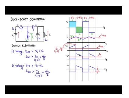
So, now this is Q and this is d let us write down the ratings for Q and ratings for D, the V CEO rating of this when the switch is off. Collector is at V i potential and the emitter the diode is free, the diode is conducting freewheeling during that time the emitter will be connected to minus V naught.
