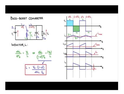
Let us now try to find the values of the components inductor first, then capacitor and then we will try to identify the switches and the ratings. So, first the inductor L, so let us look at the inductor current waveform we see that the inductor has a change delta i L I will call the delta i L like before in time dT S and another delta i L change during the 1 minus dT S period.
