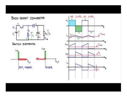
Let us now select the switch elements for the single pole, double throw switch. Considering the switch elements now, let us find out what is the static switch requirements? Static characteristics of the switch; now we will take T 1 P and T 2 P one after the other and see how the static characteristics for the switch looks like v T 1 P on the x axis, i T L p on the y axis.
