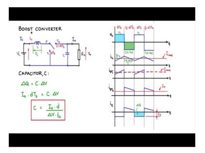
Next let us find out the value of the capacitor C, for that we have to look at the capacitor current waveform and we know from amp second balance that this area the top portion of it above the 0 line and the bottom portion of the area below the 0 line, they should match.
