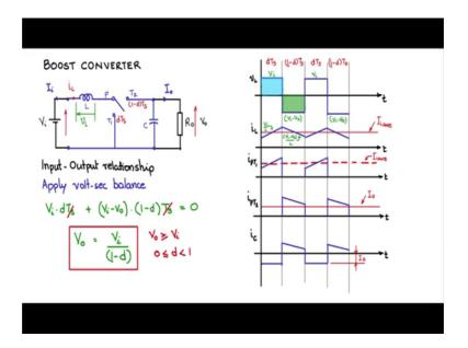
Consider the boost converter circuit. We have this inductor, single pole double throw switch and the capacitor. Let us see how it operates and the various waveforms. Let me mark this I naught current flowing through the output load resistor, I in current flowing through the input source V i. Let me mark the voltage across inductor is the voltage across the inductor V L with the common point the probe placed here and the measuring point the probe placed here.
