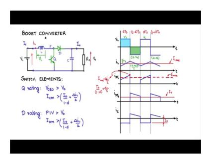
So, let us clear up this is called Q and this is D. So, this becomes the complete topology of a boost converter with the semiconductor switches in place. What are the ratings of Q and D?
