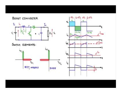
Now, let us select the switches for the single pole double throw switch and find out the ratings. So, the switch elements like we did for the bug convertor, we will use the static
