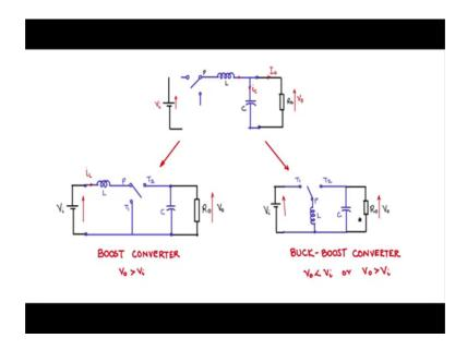
Consider this Buck Converter topology here we used we used one SPTD switch single pole double throw switch 1 inductor and 1 capacitor, one of each of these components we can have 2 other configuration. So, let us just take only those parts see Vi will be on the inputs side the outputs side V naught we need to have a capacitor on the output side to filter to get a filtered V naught, so the capacitor will always be on the output side.
