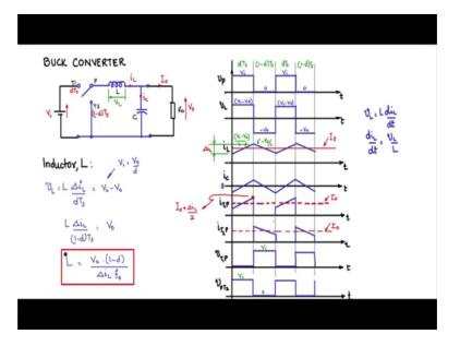
The Buck Converter has 3 important components to be designed or rated, one is the single pole double throw switch the other one is the inductor and the third component is the capacitance. Now let us take one by one let us take the inductor. So inductor L value how to find the value of L? We will use the Faraday equation VL is equal to L delta L by delta T L d iL by d T. Now we see that in the inductor current waveform it is a straight line linear because the rate is constant.
