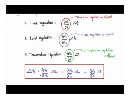
Overall, if you put all of these together, you can get the overall output voltage regulation or delta V naught at the output is delta V naught, the change in V naught with respect to line into the amount of line change deviation. Keeping now this is keeping load and these values keeping load and temperature constant plus you have the effect of change in V naught to the changes in I naught into delta I naught. Here you are keeping line voltage constant and temperature constant.
