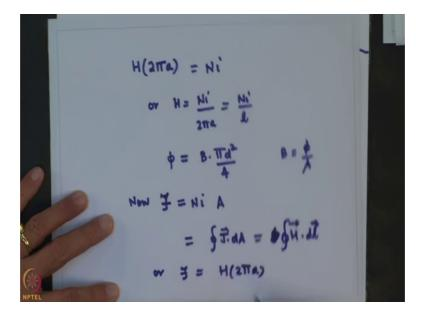
Assuming that, d is much much smaller than A. We can write H into 2 pi a which is nothing but, the mean flux path length is equal to N into i or H is equal to N idvided by 2 pi a is equal to Ni by I. L is the mean magnetic flux path length. Since, a is much larger than d, it is to assume that the flux density B is uniform across the cross section of this plastic torus.
