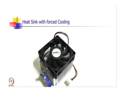
The second slide shows, a component which is mounted on the heat sink along with a fan which is used for forced cooling. In several applications a fan is required for forced cooling apart from a heat sink.
