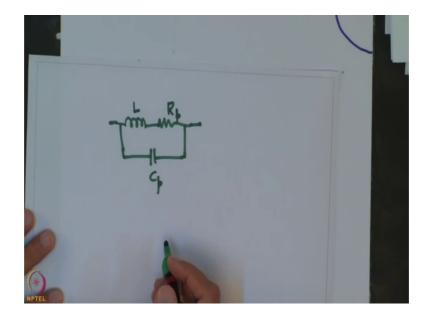
The equivalent circuit of an inductor maybe drawn like this; so this L is the main inductor, but along with it there is a parasitic inductor Rp and a parasitic capacitor which is because of the inter turn capacitance Cp. And whenever we are considering the inductor we must consider the effects of these parasitics. So, that we know that the operation of the circuit where this inductor is used will not be affected by these parasitic components.
