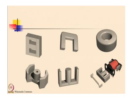
There are various types of course, the various types of geometries which you can see on the left side top is laminated low frequency pour that is used for low frequency applications. Typically this is a metal, which is made of silicon steel or which is also called transformer steel for our regular low frequency transformers and inductors this is useful. What you see in the middle on the right side in the top row is a C type core.
