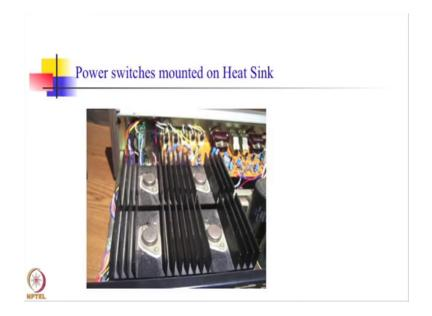
The slide shows, the power devices mounted on the heat sink. You can see very clearly the fins which are actually provided to facilitate the easy passage of heat into the ambient.
