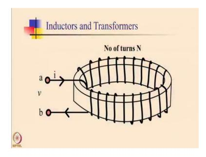
The other important components of a power electronic system are the inductors and the transformers. The inductors work as filters or snubbers or energy storage elements; which are fundamental to the working of certain power converters. The transformers are used for voltage or current transformation and galvanic isolation ok.
