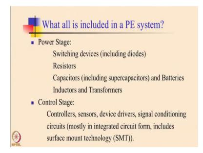
Welcome back to Fundamentals of Power Electronics. Any power electronic system consists of two stages, a power stage and the control stage. The power stage, which is a very common name given to the power circuit or the power electronic system yes. So, it has the switching devices inputting diodes it has got resistors; also whether we want them or not we do need resistors for various applications.
