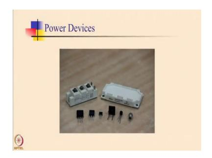
Here, you see the various packages in which the power devices are available. So, what you see in the you know towards the back side are two IGBT modules. So, these are fully controllable devices meaning that they can be controlled; through their control terminals whether its turning on or turning off they can be completely controlled through this controlling terminal.
