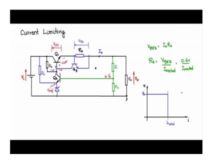
Let us create some space here to introduce some components here. And let me introduce a resistance in this fashion. And across the resistance let me connect the base emitter of a transistor, and the collector the transistor is connected to this point.
