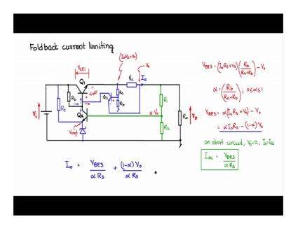
Now, let me explain this. Let me remove this portion make a bit more space and I will put the resistance R s here. And from this point, I will tap a voltage divider to ground. And to the centre point of that, I will connect to the base of the BJT Q 3. So, the collector I connect it in the same way and the emitter also I connect in the same way to this point output point.
