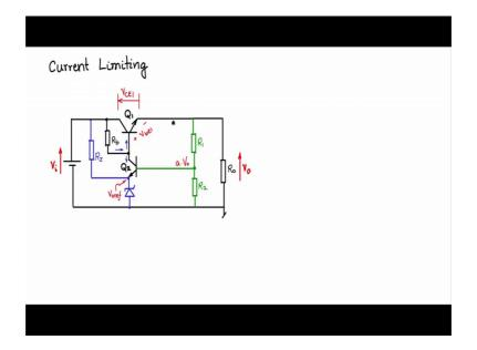
Let us now discuss how to provide current limiting for the series regulator circuit. Now, consider the series regulator circuit and let us introduce some components here such that we limit the current under, overloading or short circuit conditions.
