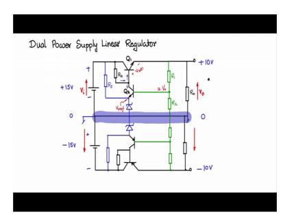
So, let me redraw the flipped negative regulator. So, let me redraw that. So, I am redrawing with the ground flipped compare, now this is a p-n-p I am replacing the n-p-n with a p-n-p, I am replacing this n-p-n with a p-n-p, but now the regulator is flipped compare with what we have [dawn/drawn] drawn previously this is R naught, these are
