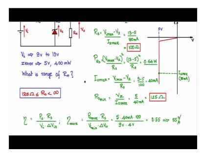
What is efficiency? You can calculate the efficiency of this to complete the understanding. So, efficiency is we have found out that V naught into R s by V i into delta V io or the delta input output differential.
