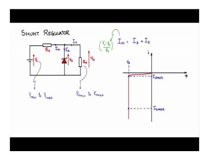
Let us now discuss the Shunt regulator circuit. So, let us draw the input unregulated voltage V i, it contains a series component here and a shunt component here, it is a Zener diode and the load. So, this is the structure of a shunt regulator. The hero of this is this Zener diode. This is V i, the unregulated V i, we will call this as R s, this is V z and this is the load resistance R naught and you have V naught and V naught is equal to V z.
