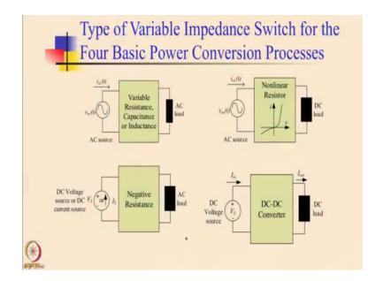
So, just to quickly summarize that you know you can actually have AC to AC conversion when you can have a variable resistance or capacitance or inductance. We saw the example of a magnetic amplifier where it was an inductive impedance you know that was switched from the maximum value to the minimum value, and vice versa to control power.
