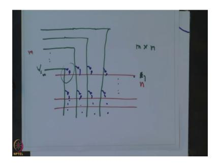
So, these are the m input lines and with the red pen let me just draw the output lines. So, these are n output lines and m input lines, ok. Right now, they are just actually plays in this crisscross fashion. Now, if I connect at each of the points where the input and the output lines meet one switch, ok.
