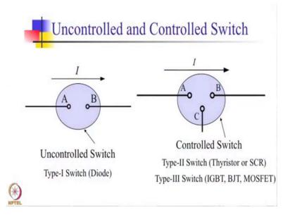
Uncontrolled and controlled these are the two types of switches, when we talk of about diodes these are uncontrolled switches. And we call them type one devices, when we talk
