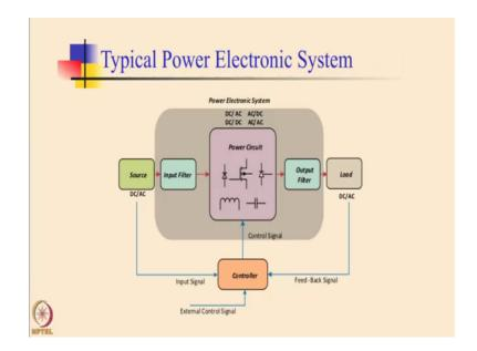
Now, very briefly now we will come to this point again we will just briefly see how a typical power electronic circuit looks like, ok. So, here is a typical power electronics system, ok. So, what you see at the heart or at the center of the system is a power converter and as we have been every, as we have seen before it is able to change the form of electricity.
