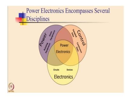
And actually, we will see that the power electronics borrows concepts from the power engineering field, the control engineering field, as well as the electronics engineering field and that is how the entity of power electronics comes into being, ok. So, you can see that in this picture power electronics is shown as an overlap of the three main sub disciplines of electrical engineering, the power, the control and the electronics engineering.
