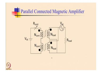
Now, here is an example of you know an inductive switching. So, what you see here on the right side is a load which is supplied by a V ac or source and on the left side we have coupled a DC source along with a control resistor. So, actually you apply a DC current into this coupled inductors. So, you can see here these coupled inductors. You are actually trying to inject through this a DC current and in the process what we do is we saturate the core.
