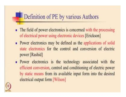
Likewise, there are many other definitions, one of the definitions that I will like to quote is from Professor Wilson, which says power electrons is a technology associated with the efficient conversion control and conditioning of electric power by static means from its available input form into the desired electrical output form. So, this is what is the definition given by Professor Wilson in one of his papers.
