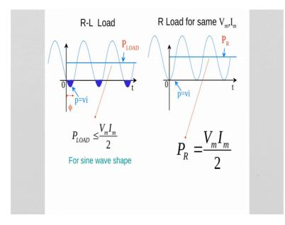
And P load is less than P R, it is less than V m I m by 2 because of this negative part.
