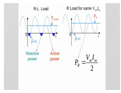
Now, let us find out the powers the instantaneous power curve we know is like this. There is some negative portion here for the R-L load and for the R load there are no negative, there is no negative portions. This is the average P R, this is the average P load for the unknown R-L load.
