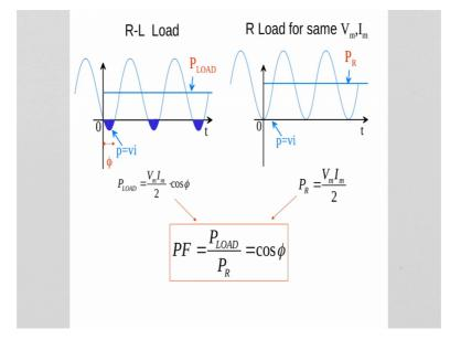
And if it is a sinusoidal case we know that for sine waves P load is V m I m by 2 cos phi where this is phi. So, we now apply our definition of PF is P load by P R any wave shape and for this special case of a sine wave you will get cos phi. So, it verifies that the definition that we have made as a measure of closeness to a pure resistive load any load, any unknown load, measure the closes to a resistive load will provide you the power factor value.
