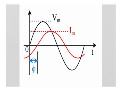
Consider an oscillogram x axis is time and let us place a voltage waveform on this is a voltage waveform and it has a peak amplitude of V m and superimpose a current waveform with an arbitrary delay meaning an R-L load and that delay is phi. And let the current have a maximum value of I m. So, the voltage wave shape in have the equation V m sin omega t, the current wave shape will be having I m sin omega t minus phi.
