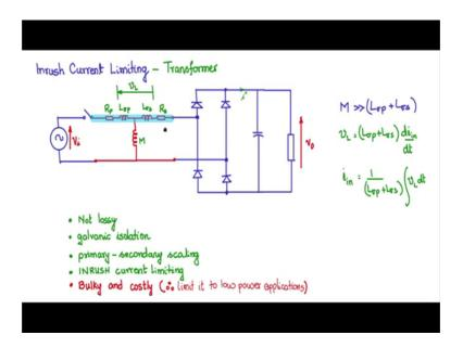
So, what we shall do? We shall replace this transformer with its equivalent circuit. I will take n is equal to 1 for now it really does not matter even if n is other than 1. So, we will replace it by a transformer t network equivalent where this is the mutual inductance M, this is the primary leakage, secondary leakage or primary or secondary; so, the winding resistances.
