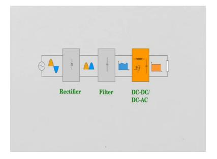
A typical power electronic system will look something like this. You have the AC source here it gives you an AC voltage. So, voltage source 230 volts and the power flows into rectifier which is normally a diode bridge rectifier get a rectifier output passes through a filter and the filter filters out the output voltage to a filter DC. The filter can be an LC filter or just AC filter and most cases it is just only AC filter.
